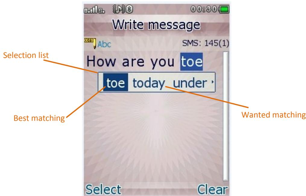
The selection list is a visible feature of the XT9 input method, in which the words appear in a horizontal list just below the inserted text. When the user enters characters, the XT9 examines available databases for the words that best interpret the characters entered.
